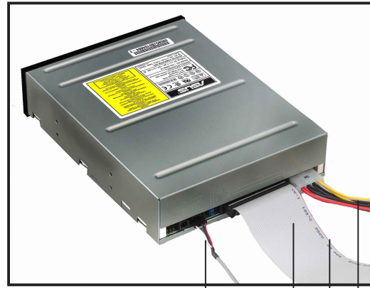
CD-ROM audio cable IDE ribbon cable Red stripe to pin 1 Power cable
